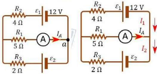
$$V_a + \Sigma \Delta V = V_a \rightarrow \Sigma \Delta V = 0$$
